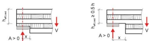
Figure 13: Verification of notches in CLT panels [14]
