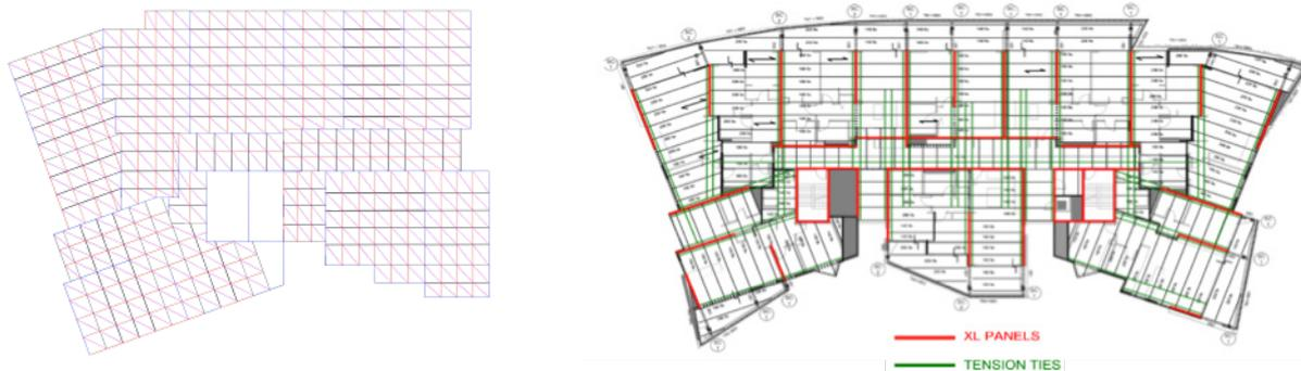
a) Equivalent Truss Model (only the left part of the diaphragm is shown)
