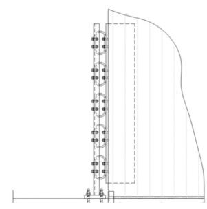
Figure 5: UFP hold down / energy dissipater.
