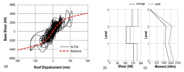
Figure 11: Analysis Results. (a) Force-displacement plot for record 2. Example of (b) Shear force and (c) bending moment envelopes.
