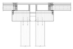
Figure 3: Double glulam beam.
