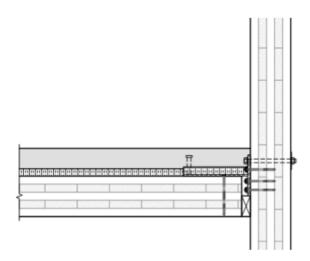
Figure 7: Concrete diaphragm connection to shearwall.
