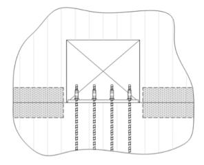
Figure 4: Post-tension rods in CLT wall (top) and rod connection and CLT splice (above).
