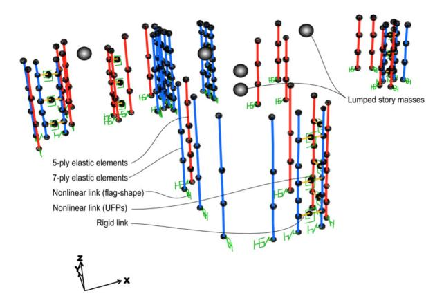
Figure 9: Model for the nonlinear response history procedure.
