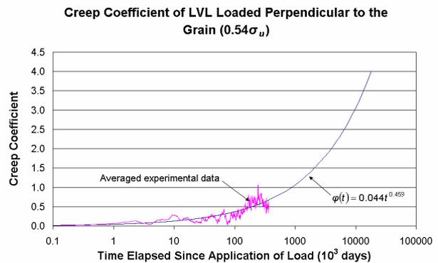
Fig. 12 Creep coefficient of LVL blocks in compression perpendicular to grain in an uncontrolled, heated, indoor environment (extrapolated to 50 years)
