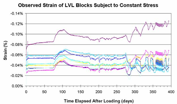
Fig. 9 Observed strains of LVL blocks subject to constant stress ( $0.08\sigma_u$ ) parallel to the grain in a controlled environment
