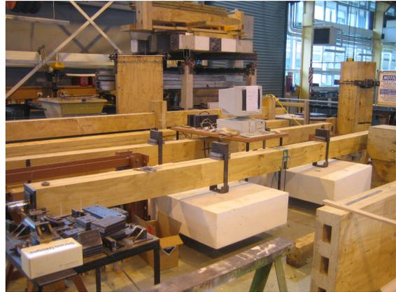
Fig. 7 Beam specimens in the uncontrolled environment tested in bending (in the foreground: prestressed specimen)
