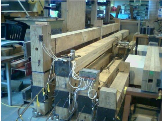
Fig. 6 Frame (on left and on the floor) and beam (on top of the second frame specimen, from left) specimens in the uncontrolled environment. On right: beam specimen loaded in bending
