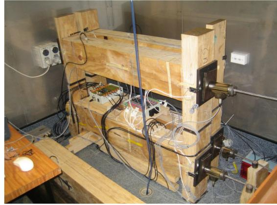
Fig. 5 Frame specimens in controlled environment
