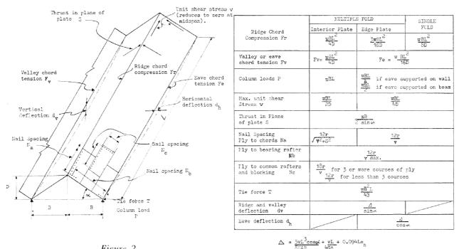
Figure 2 Figure 2. Forces in a simple span Folded-Plate roof under uniformly distributed live load.
