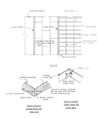
Figure 1. Folded-Plate construction detail.
