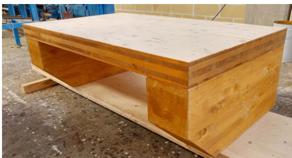
Figure 11: Mock-up of a roof portion (secondary beams and Cross-Lam) aimed at the study of the waterproofing covering and interference with joints and connections on the roof.
