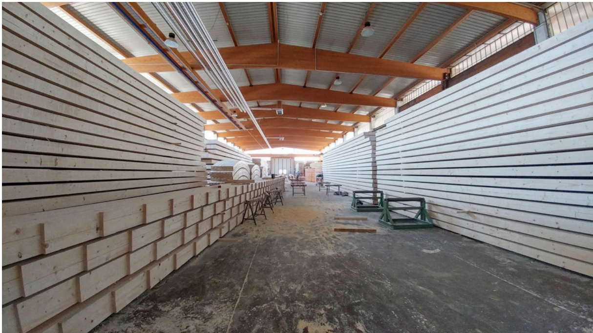
Figure 12: Factory of Rubner Holzbau Sud a Calitri (AV) Italy, glulam beams ready to be pre-assembled.
